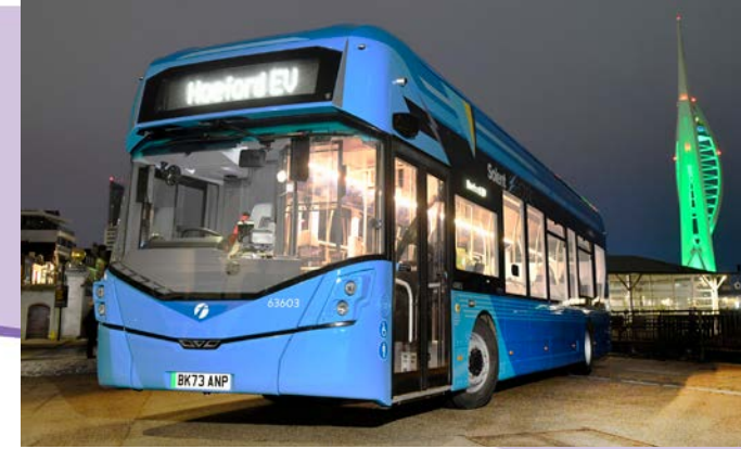
Battery-electric buses, such as this example built for First Bus in Portsmouth by UK manufacturer Wrightbus, are key to the industry's drive to decarbonise its networks.
